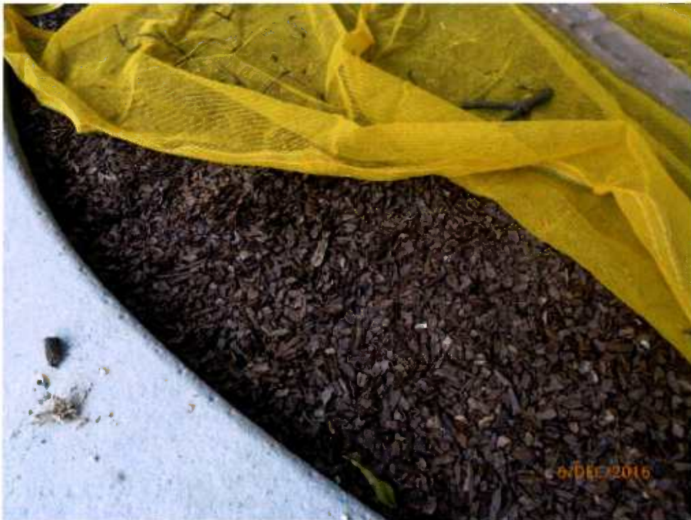
Fig. 11 Size of the pine bark mulch is too small, not up to ASD Spec. required standard.
